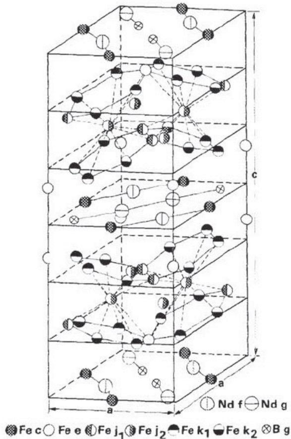
FIG. 1. Tetragonal unit cell of the  $\text{Nd}_2\text{Fe}_{14}\text{B}$  structure.
