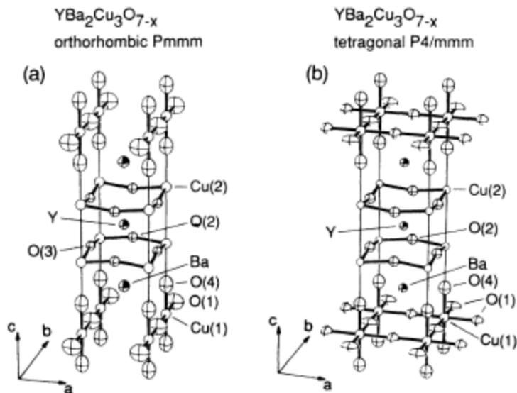
FIG. 1. (a) Orthorhombic and (b) tetragonal structures of  $\text{YBa}_2\text{Cu}_3\text{O}_{7-\delta}$ . In the tetragonal structure (b) the different atom symbol for the O(1) site is used to indicate that this site is not fully occupied.
