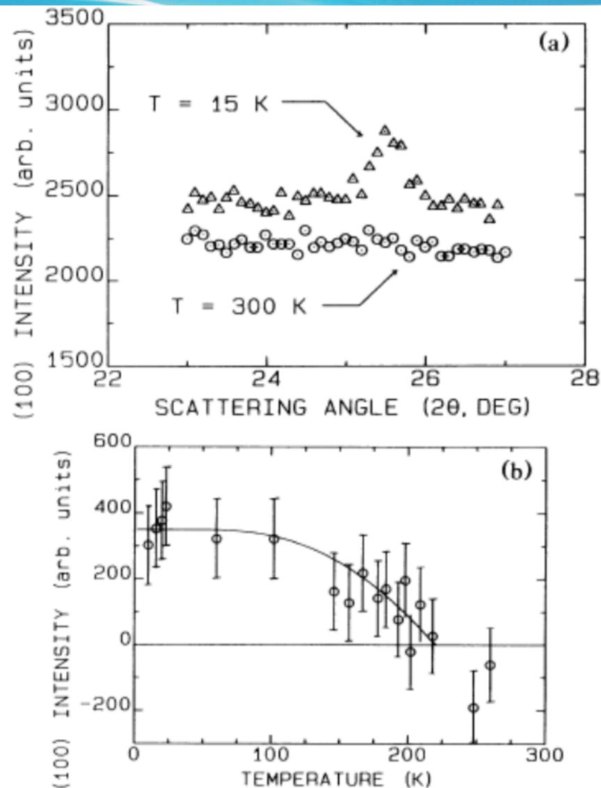
FIG. 2. (a) Intensity vs scattering angle  $2\theta$  for neutron powder scans of the (100) peak region at 15 K and at room temperature. (b) (100) peak intensity vs temperature. The line is a spin- $\frac{1}{2}$  magnetization curve for  $T_N = 220$  K, calculated from molecular-field theory.
