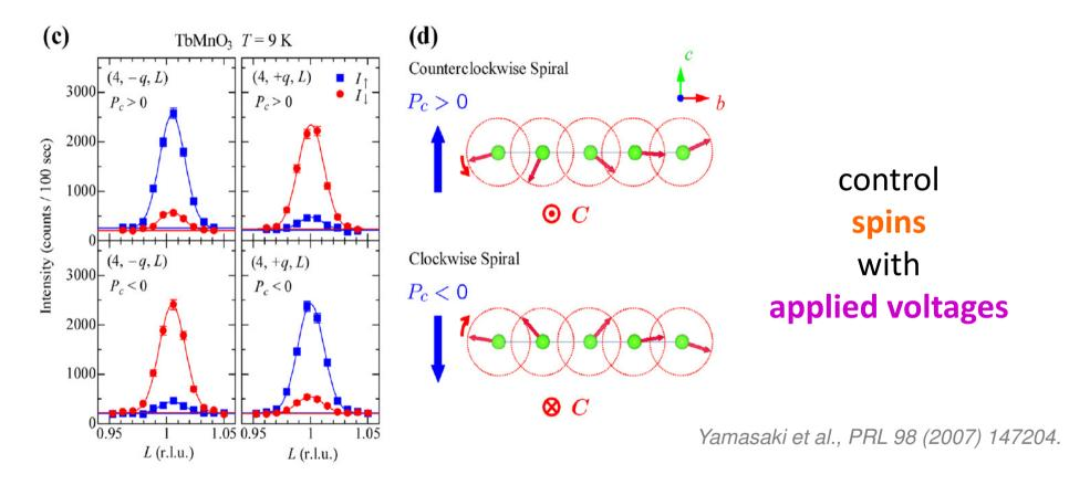
Essential: Neutron Diffraction with polarization analysis was used to determine the helicity of the magnetic spiral
