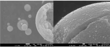
Hollow sphere aggregates made via the spray pyrolysis method – diameters ~ 70nm
