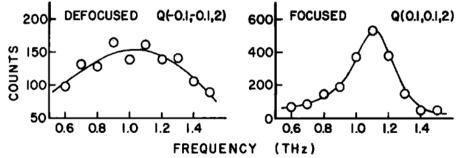
FIG. 12. The neutron groups corresponding to a T[110] low-lying acoustic phonon in Cu with **q** taken, respectively, in the clockwise and counterclockwise sense from the [002] reciprocal lattice point.
