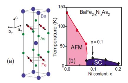
Polarized inelastic neutron scattering was used to show that the neutron spin resonance below Tc in superconducting BaFe1.9Ni0.1As2 (Tc = 20 K) is purely magnetic in origin.
