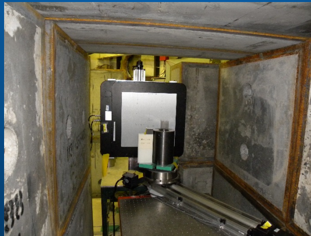
Building the dedicated flight path: L to R, Beam stop construction, the imaging location with added shielding and the open collimation beam pipe for large FOV.
