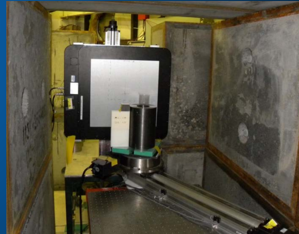
(Top) Interior of the lens coupled time of flight system and (bottom) typical flat panel CT with motion and PE1621 flat panel.
