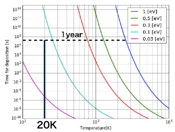
When molecules hit to the cryogenic matter surface, molecule will decrease its enegy and be trapped by surface potential.
