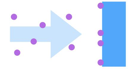
KAGRA & next generation GWD will use cryogenic mirrors. Vacuum residual gas will adhere to mirrors surface and cause refractivity change.
