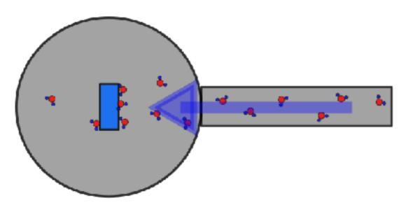
The number density of vacuum residual molecules :  $\sim 2.5 \times 10^{14} [1/m^3]$  @ P=1.0×10<sup>-6</sup> [Pa]
