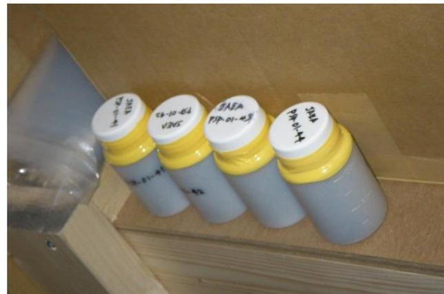
Soil samples for lab. exps. (physical property, mineral analysis, sorption-desorption exps., etc.)
