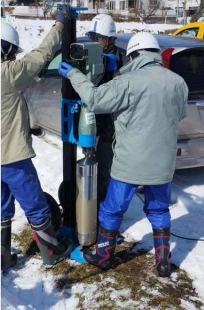
Drilling by handheld soil sampler
