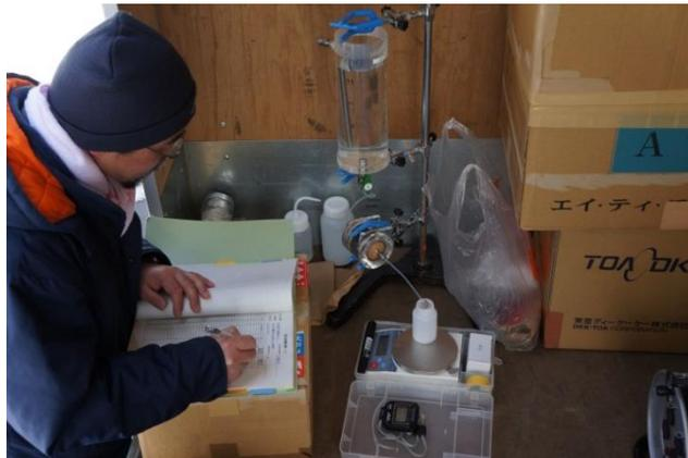
Hydraulic conductivity measurement by water head
