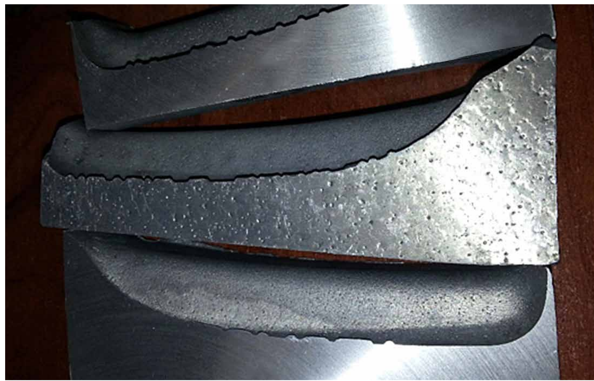
Figure 1. Material before HIP (in the middle) and after HIP (top/bottom).
