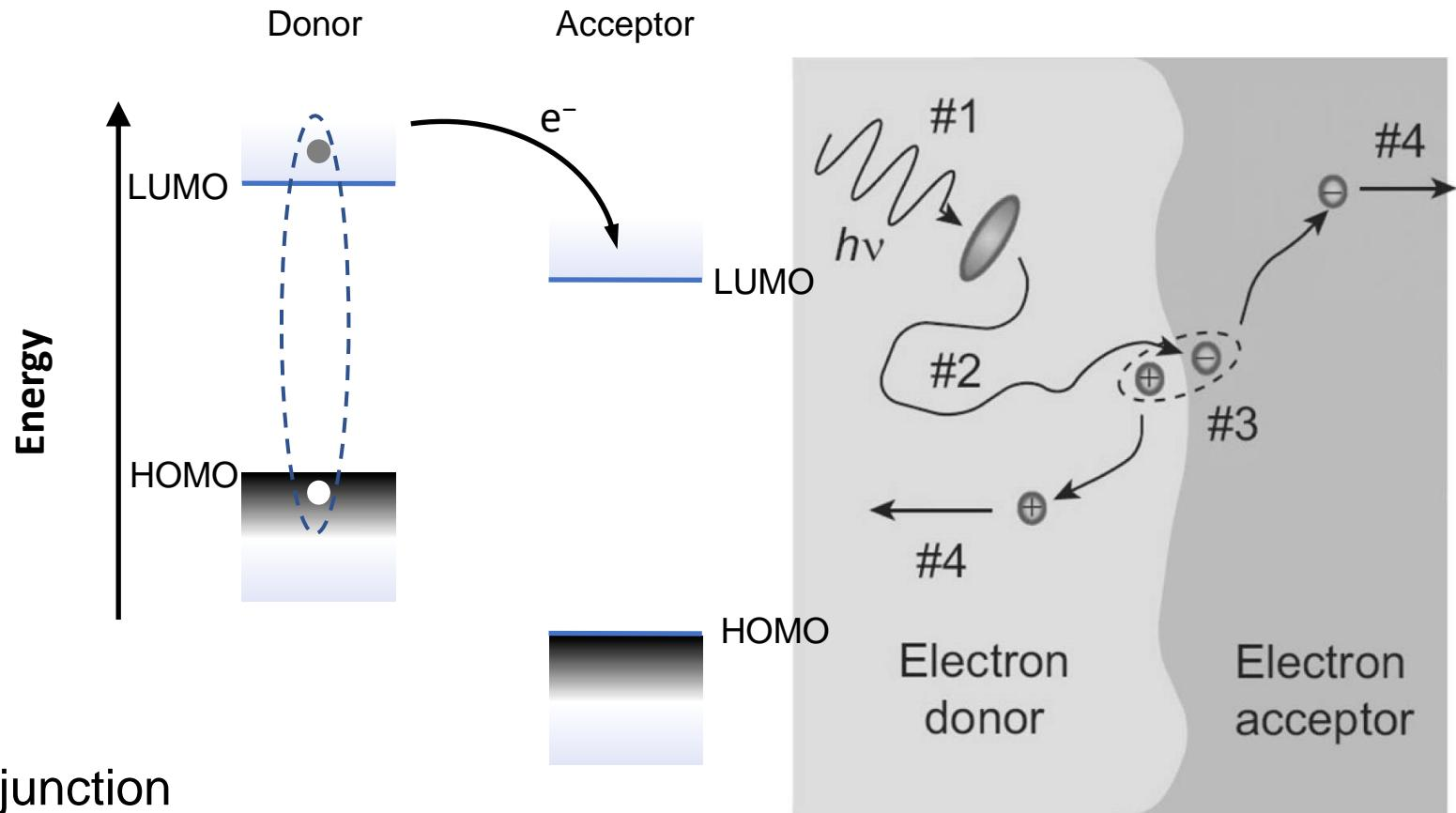
A sufficient difference in the HOMOs and LUMOs of the donor and acceptor materials is required. The “acceptor” has the higher electron affinity (deeper LUMO).
