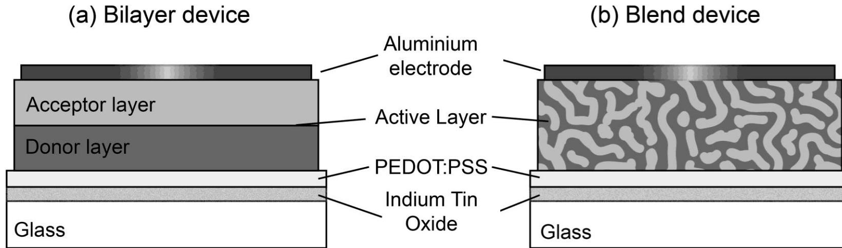
Solution is the “bulk heterojunction” which is a nanostructured blend of donor and acceptor materials.
