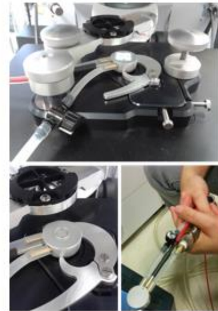
(B) Temperature-controlled hybrid macro ATR-FTIR
