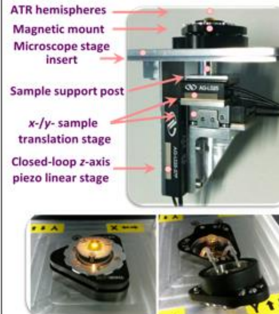
(C) Soft-contact piezo-controlled macro ATR-FTIR (chemisorption)
