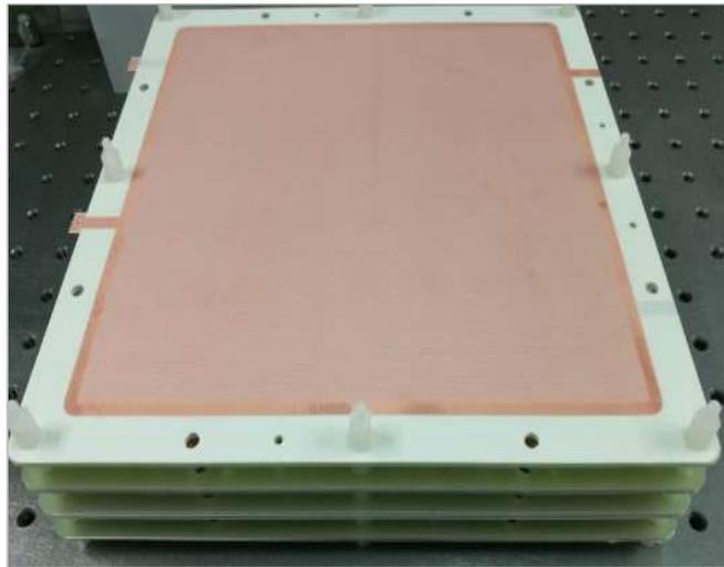
Large-area scintillation detector ( $^6\text{LiF/ZnS(Ag)}$ )
