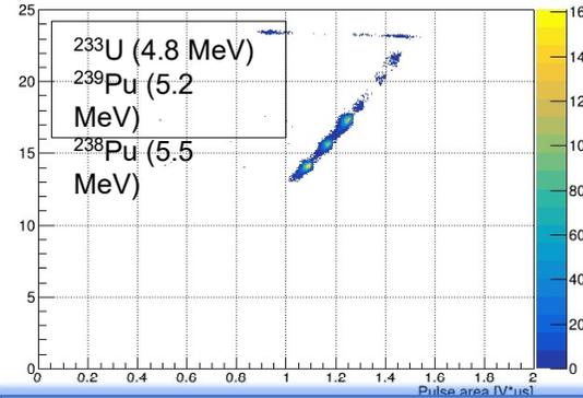
**2D plot of pulse width versus pulse area and their axis projection spectra for alpha particles from <sup>233</sup>U (4.8 MeV), <sup>239</sup>Pu (5.2 MeV) and <sup>238</sup>Pu (5.5 MeV) source. The pulse width and pulse area spectra reflect those of the track range and energy. The separation between peaks are more than 8 sigma.**
