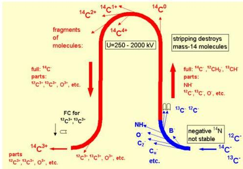
**BINP AMS provides reliable separation of a pure beam of radiocarbon ions from the accompanying ion background. But that technique can't separate the isobars - different chemical elements having the same atomic mass. The typical example are radioactive isotopes <sup>10</sup>Be and <sup>10</sup>B.**
