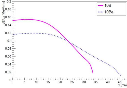
**The idea is to use the TPC with low pressure gas filling to measure track ranges from different ion species.**
