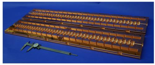
Integrated Damping Slot Damping with NiChrome Coating
