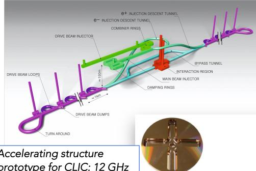
Accelerating structure prototype for CLIC: 12 GHz (L~25 cm)
