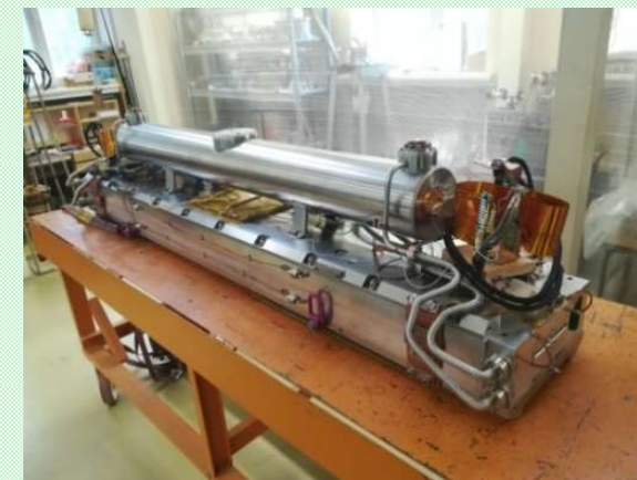
The undulator is assembled with LHe volume
