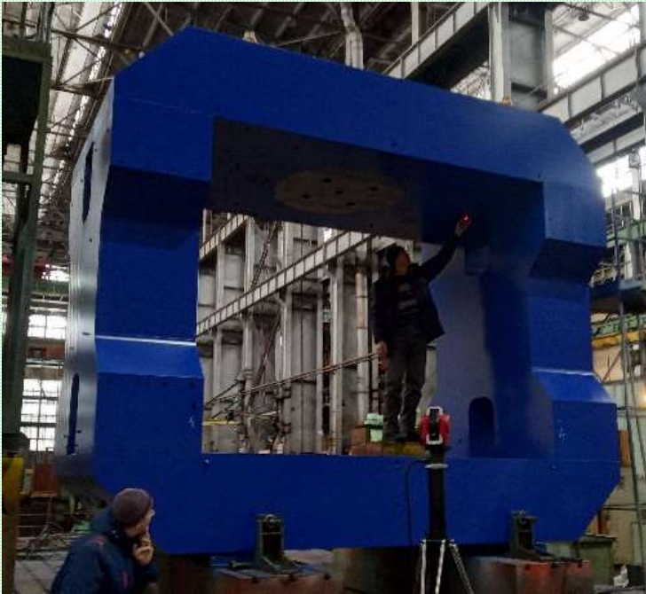
Iron yoke was manufactured in December 2021. The geometry measurement procedure is shown here.
