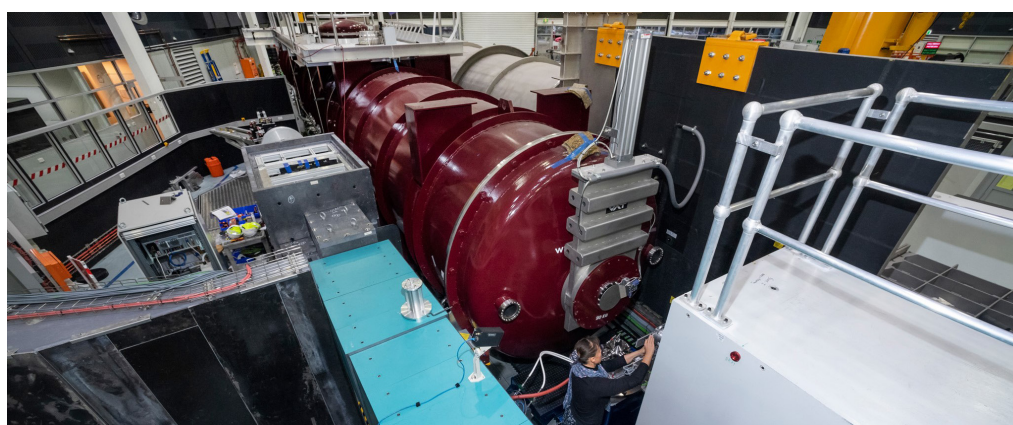
The detector tank and sample area of the Bilby SANS instrument
