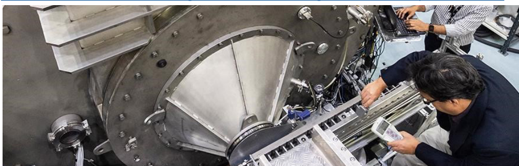
The sample area of the Quokka SANS instrument
